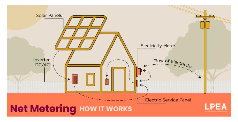
**NOTE:** The meter can only measure electricity that flows across it, either into your home or onto the grid. The meter does not know how much energy your solar system produced or how much energy your home consumed, only how much flowed either to or from LPEA's grid. The energy your inverter produces will first be used in your home and only excess unused energy goes back through our meter to the grid. This is why the amount of energy your inverter produces does not match your Net Generation.
