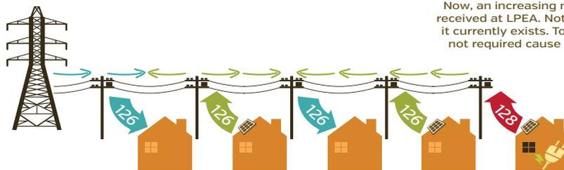
Now, an increasing number of requests for solar installations are being received at LPEA. Not all can be accommodated with the electric grid as it currently exists. Too many solar systems generating power when it is not required cause the voltage to go above the electrical grid's design limits, impacting the entire line.
